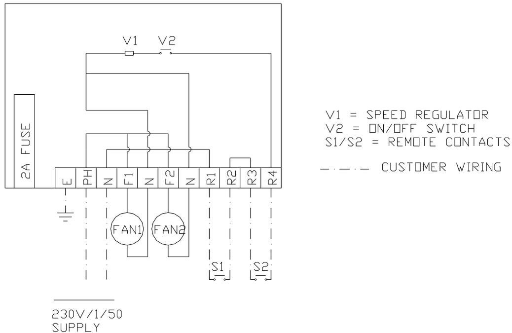
Figure 2. Wiring details DERV units
