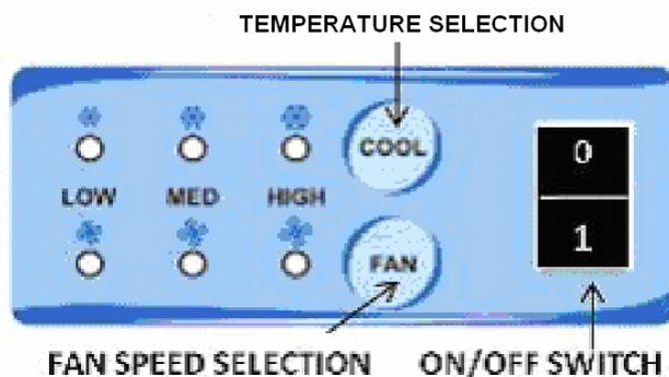
Figure 4. Controller display
