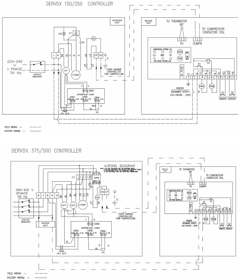
Figure 3. Wiring details DERVDX units
